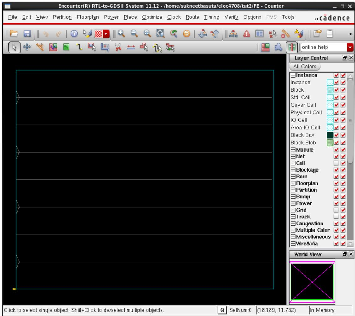
9. The next step is to specify the floor plan. We need to leave enough space so that the router will be able to place all the metal interconnects, but not so much that we waste space. We also want to have a large enough space for any buffers that might be needed during optimization. A decent number for core utilization is somewhere between 0.5 and 0.7 (The default is most likely fine).
