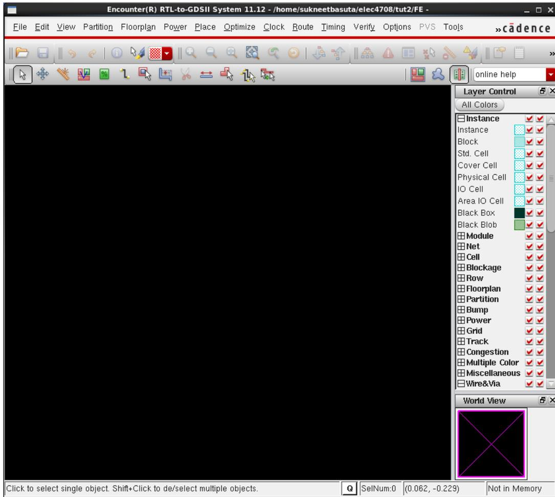
6. In encounter we now need to import the design that we saved in the synthesized directory. Go to File -> Design Import, and fill in the pop-up window as shown below (modify the file locations to suit where your files are saved). Set VDD as the Power net, and VSS as the ground net.
