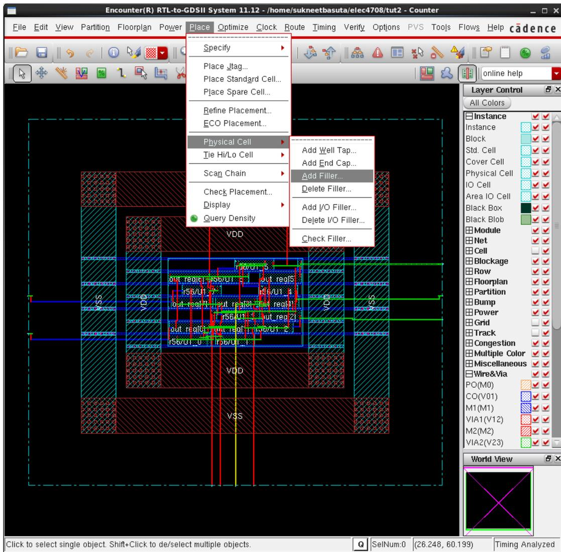
In the Add Filler window, select the DCAP and FILL1 cells and check of Mark Fixed. DCAP places a capacitor between VDD and VSS.
