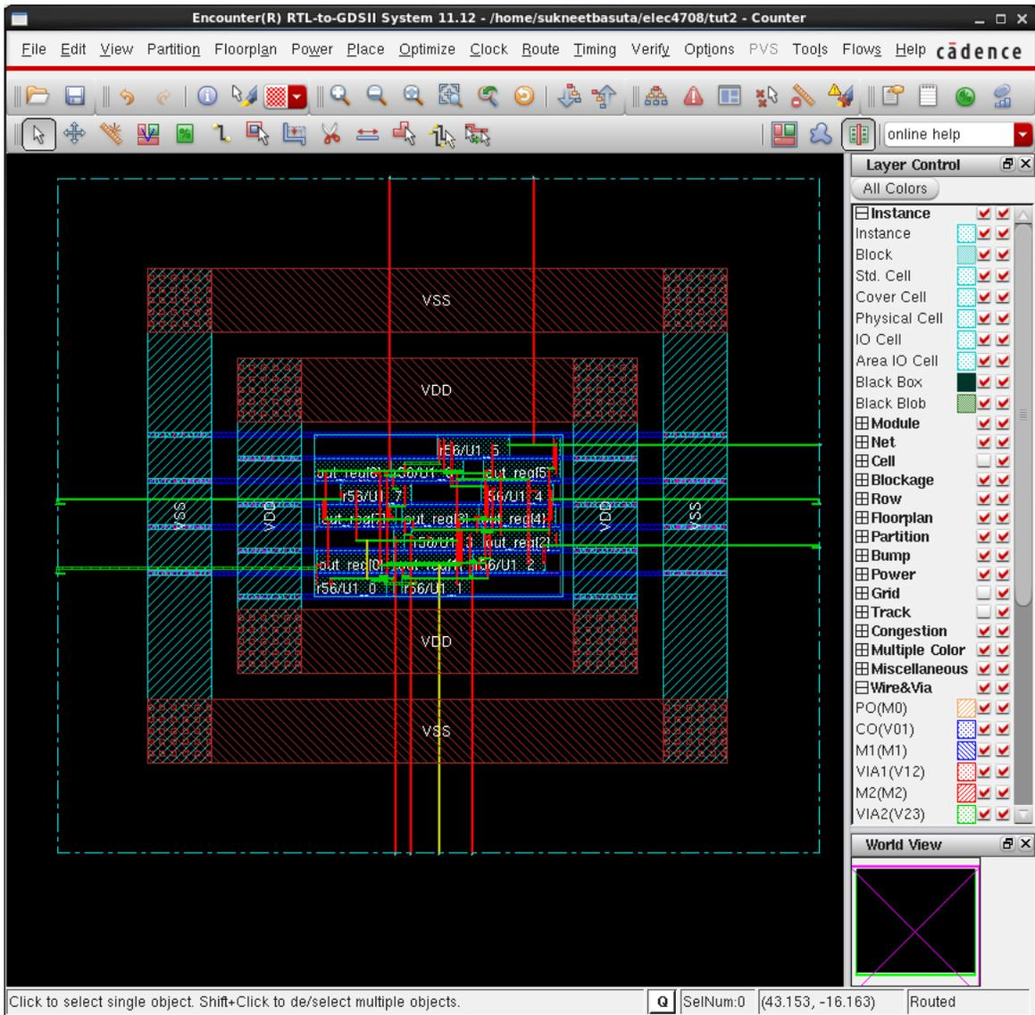
If you zoom in, you may notice that you cannot see inside the cells. If you Check the first checkbox for **Cell** under layer Control on the right, you can see inside the cells.
