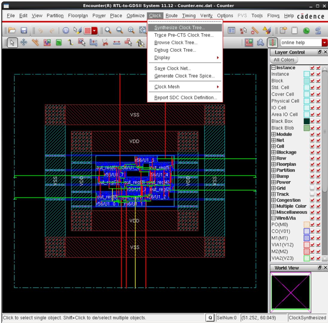
The Synthesize Clock Tree window should popup. Set the Clock Specification file to "Clock.ctstch". The rest of the defaults should be fine. Hit OK and look at the terminal to determine if it was successful.
