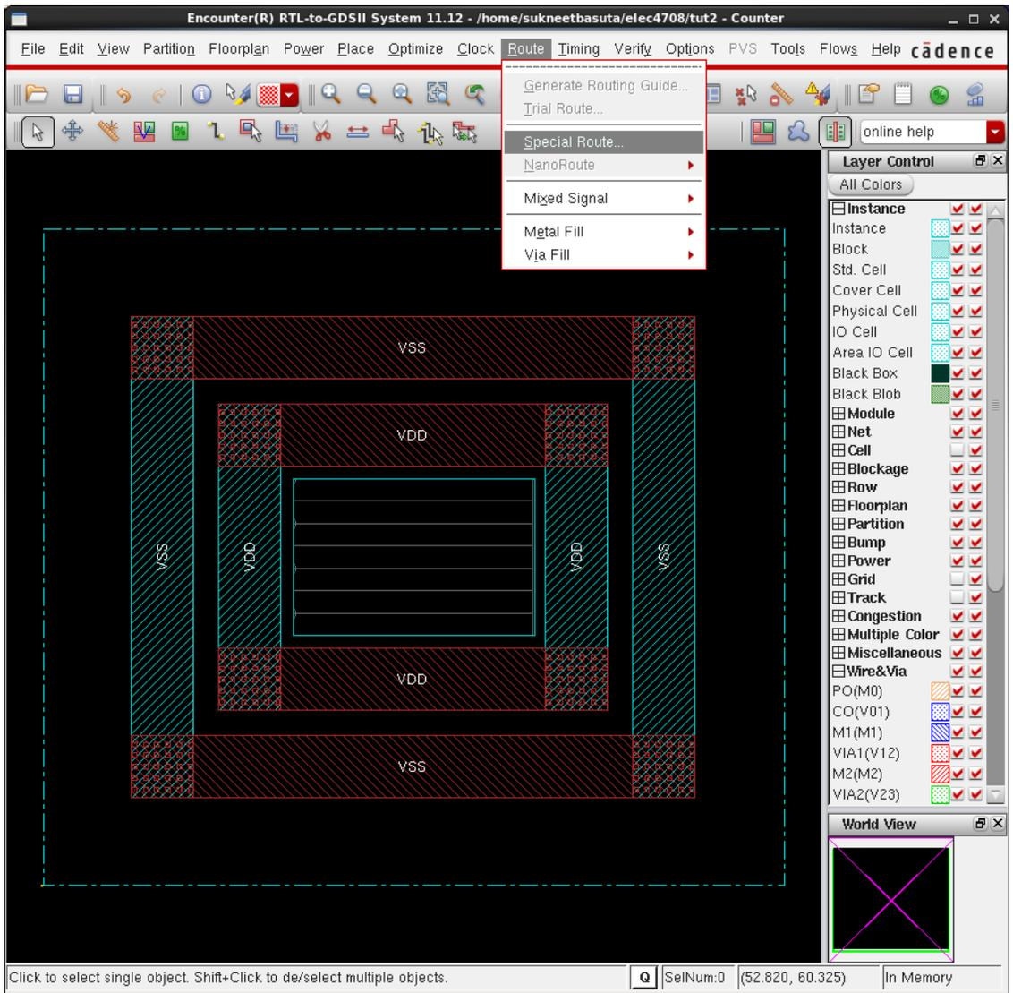
14. In the SRoute window, select the VDD and VSS nets by clicking on the “...” button. The rest of the defaults should be fine.
