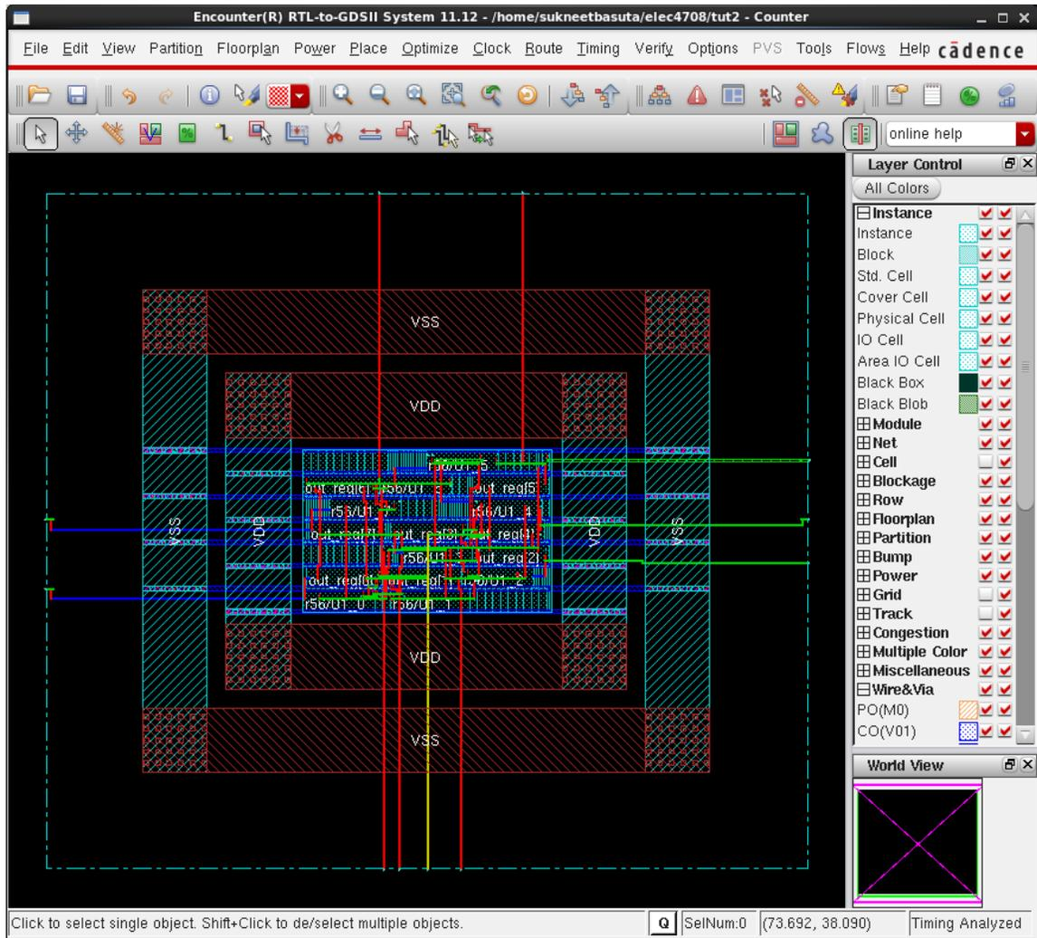
23. Now that the layout is complete, let's verify the layout. Let's verify the connectivity and geometry. Select **Verify -> Verify Geometry** and **Verify -> Verify Connectivity**. Use the default values for both cases. You will see the results in the terminal window.
