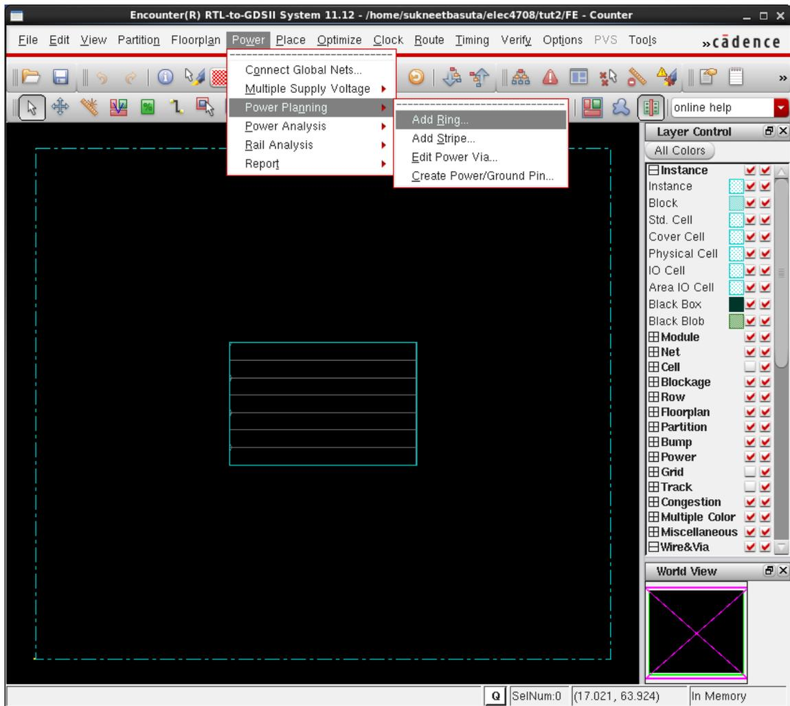
12. Select the VDD and VSS Nets by clicking on the “...” button. Make the power lines 5 microns wide and use Metal 9 for top and bottom and metal8 for left and right. Click on “Update”. Set an offset of 1 micron. Click “OK”. The width of the power lines is determined (somewhat) by the size of the chip. A much bigger design would need wider lines.
