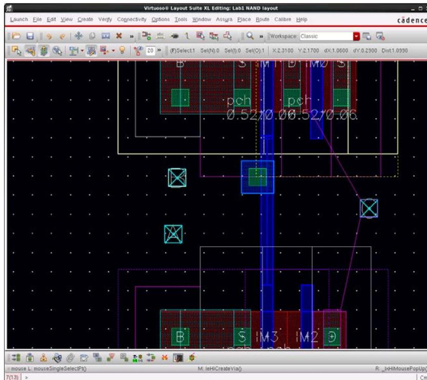
23. Wire up the rest of your layout. Using Point to Point (**Create -> Point to Point – Ctrl+Shift+P**), or manually creating shapes may help you wire up your design. (Don't be concerned if your layout is not exactly the same)
