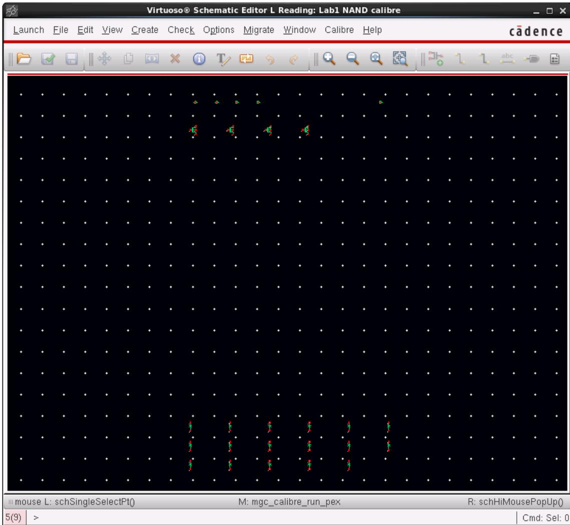
65. The schematic will look odd to you since we told Calibre to array the devices (not doing so can cause devices to overlap) and because the devices are connected by short wires and label names. If you take a closer look, you will see the 4 transistors in your NAND gate and the input pins.
