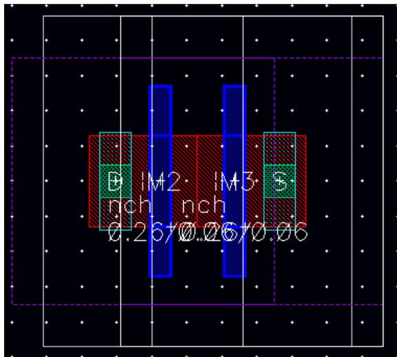
To break the chain, drag the transistors apart. Move one device to the other side, Right click the device, and select **Rotate -> Flip Horizontal**. Do this to both devices.
