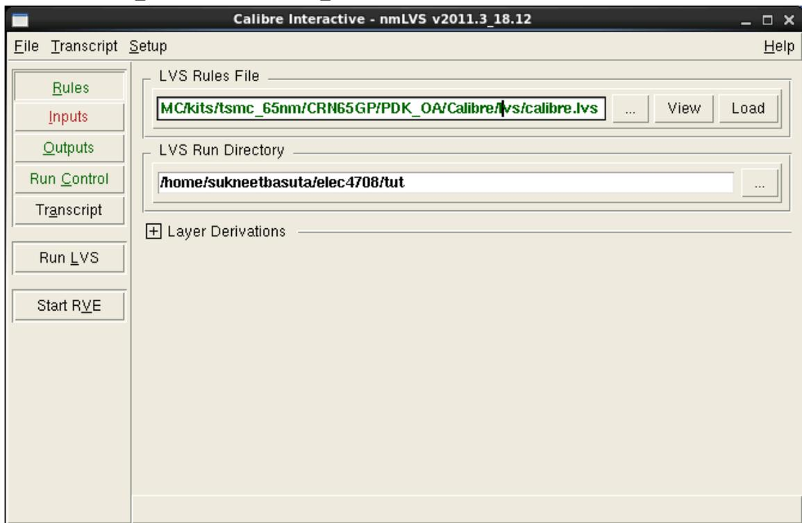
45. Select the Inputs button on the left. Then Select the Netlist tab in the middle. Check the “Export from schematic viewer” option
