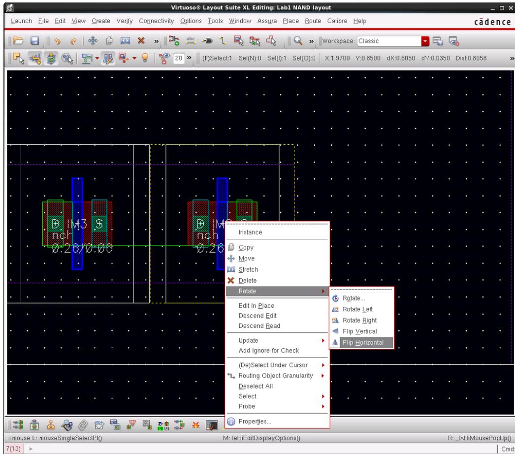
Once they have both been rotated, drag the devices on top of each other and they should chain together.
