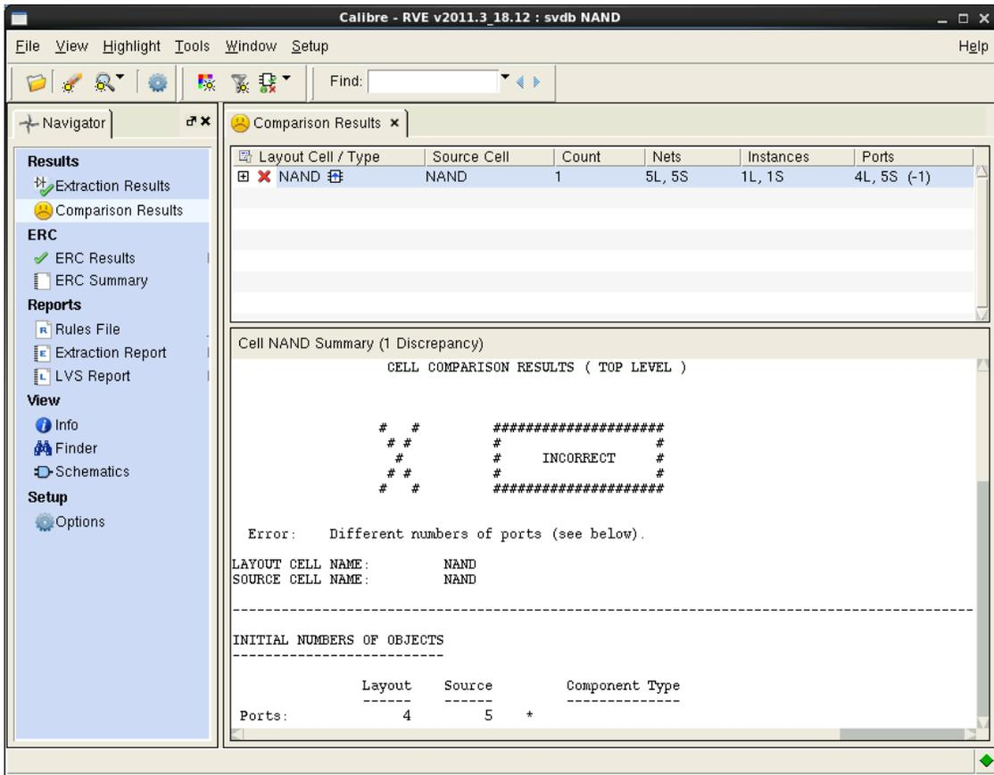
51. We can see the problem by clicking the + next to error. When you click on the expanded error, an explanation of the error will appear where the summary was. Clicking on any Red links in this area (i.e. A in the image below) will show you the schematic the LVS run got from the layout on the left and the schematic you designed the right.
