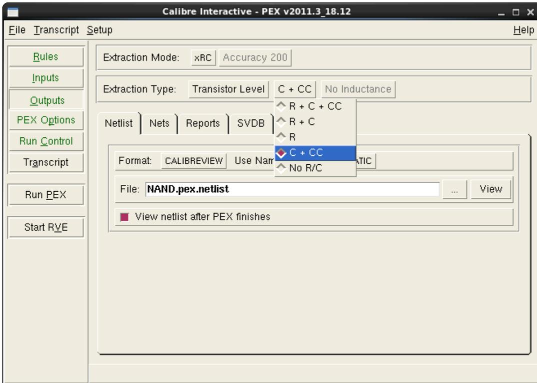
59. Select Setup -> PEX Options. The PEX Options button should appear on the left. Click it. Select the LVS Options tab, and set the Power nets (VDD) and Ground nets (GND). These should be the same as the ones you set in the LVS step.
