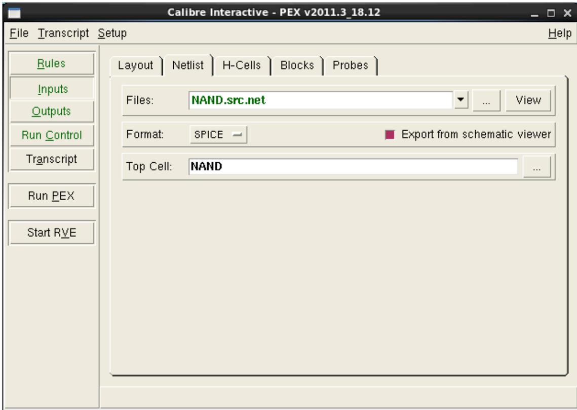
58. Since, we only want parasitic capacitances, click on the Outputs button on the left, and change the extraction type to C+CC. Also change the Netlist Format to CALIBREVIEW.
