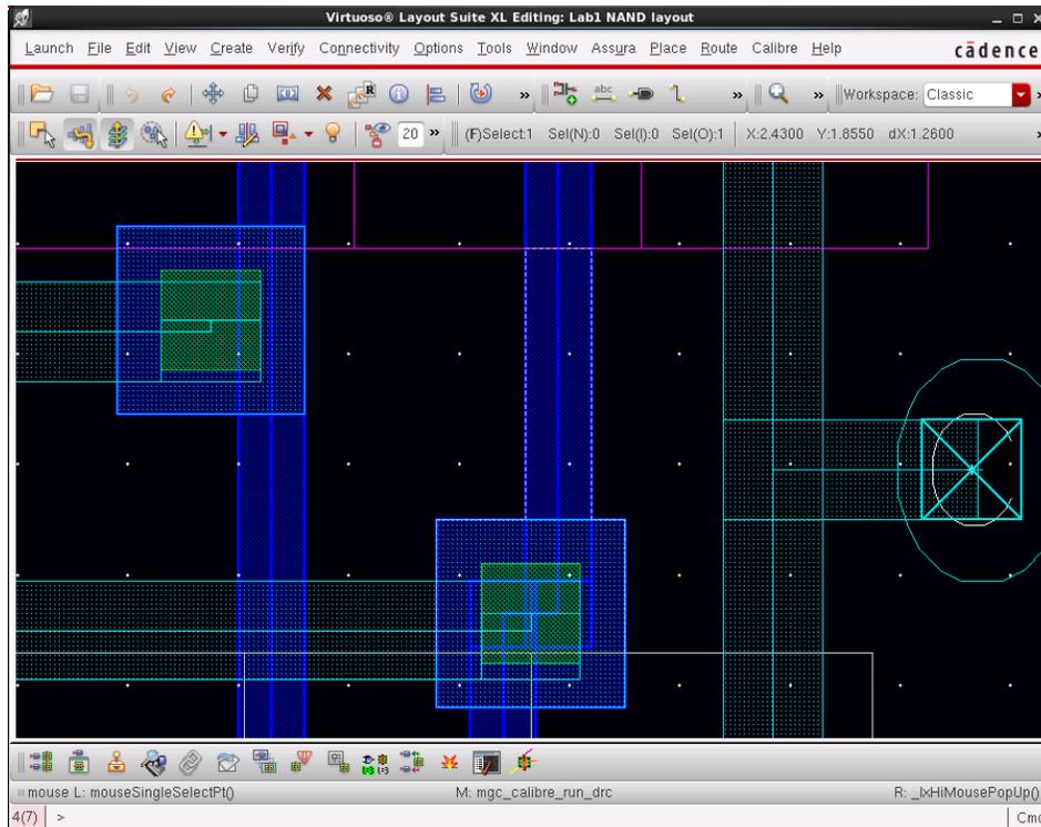
38. To fix this issue, draw a NP box under the PO layers (we are using NP since this is an N-Well process). Be careful not to overlap the PP and NP layers.
