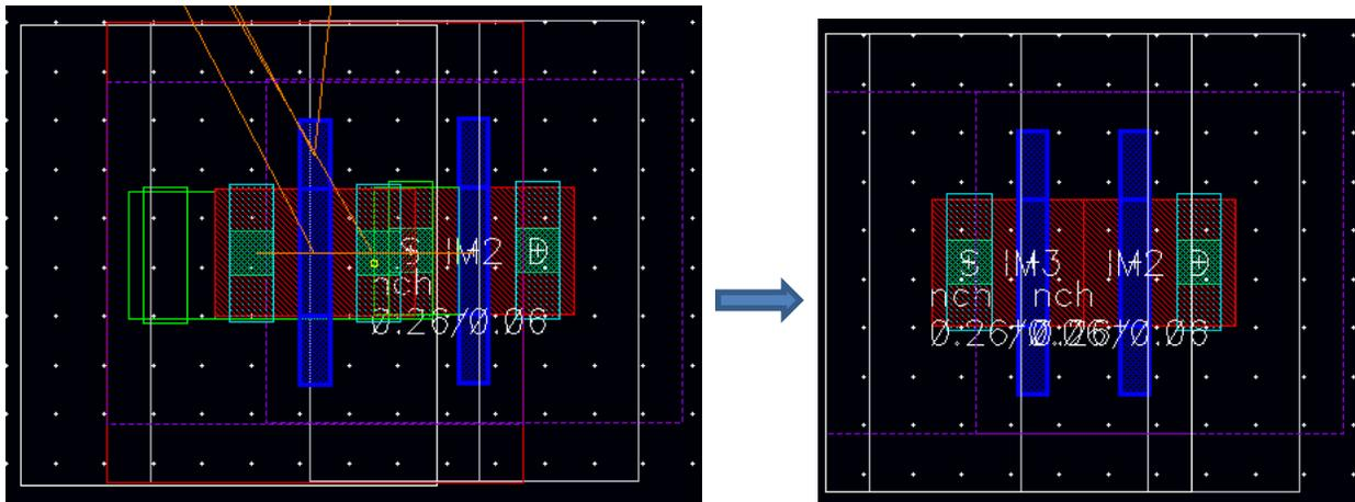
However, now the gates of the NMOS and PMOS transistors are misaligned. To fix this, change the order of the chaining of the PMOS transistors. Simply drag one transistor to the other side.
