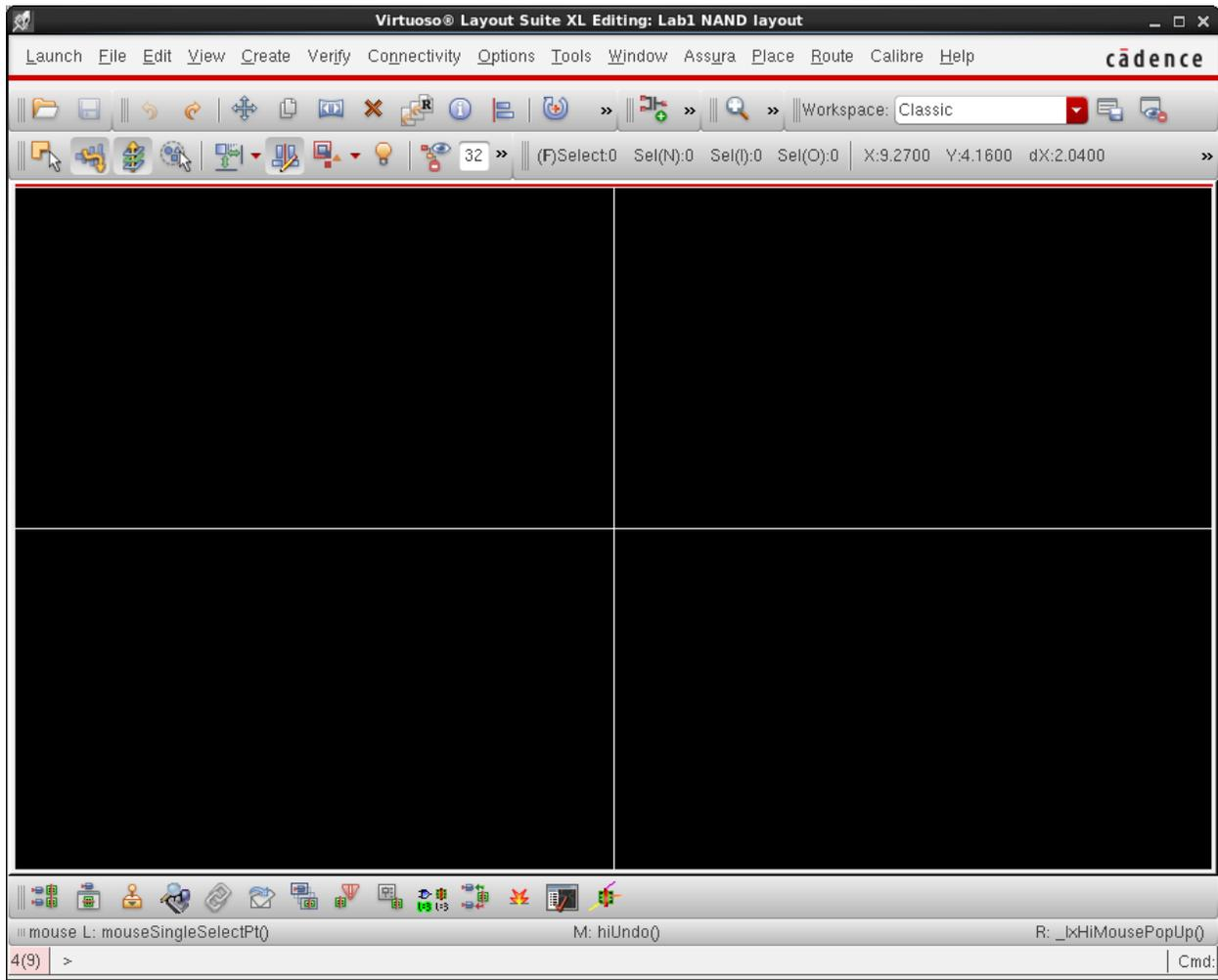
Virtuoso Layout Editor is the layout editor of the Cadence design tools. Commonly used functions can be accessed through a button bar on the top of the editor.
