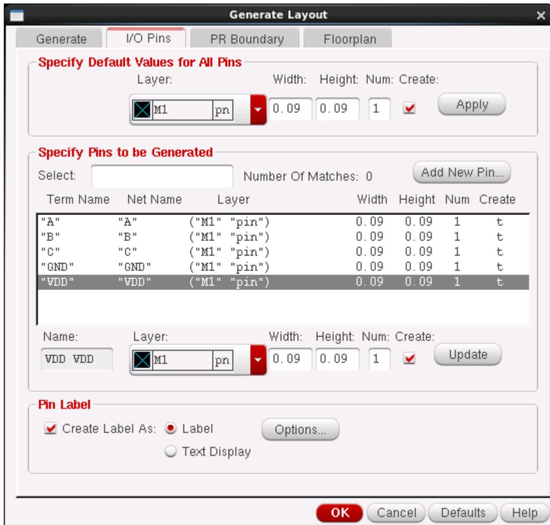
9. Check "Create label As" under Pin label and Hit the Options Button to change the text Height to 0.1. (You can also change the layer name to M1, and Layer Purpose to Pin to skip a step later, but I like to do this at the end, in case I have to change the Pin layer)
