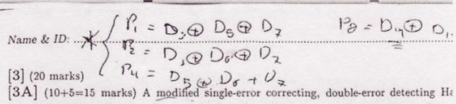
[3A] (10+5=15 marks) A modified single-error correcting, double-error detecting Ha four bits of Data  $D_3$ ,  $D_5$ ,  $D_6$ , and  $D_7$  has the following parity bit equations:  $P_1 = P_2 = D_3 \oplus D_5 \oplus D_7$ ,  $P_4 = D_3 \oplus D_6 \oplus D_7$ , and  $P_8 = D_5 \oplus D_6 \oplus D_7$ .
