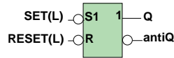
THE SYMBOL FOR THE TWO-NAND-GATE LATCH. The "1" shows that the Set dominates the Reset when both are applied at once.
