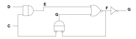
• 5.a) (10 marks) Identify the type(s) and condition(s) for the hazard(s).
