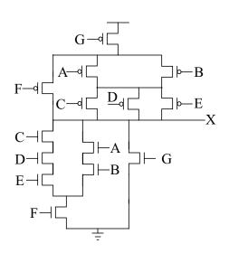
b) Topology (a) gives highest delay because it has highest parasitic capacitance at output. The following topology gives lowest delay, because it only has one PMOS and two NMOS diffusion capacitances at output.
