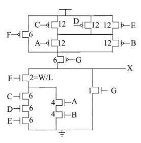
c) In (b) transistors are sized such that any NMOS path has  $(W/L)_{eff}=1$  and any PMOS path has  $(W/L)_{eff}=3$ .
