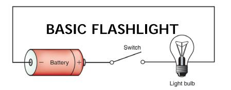
Converts energy stored in battery to thermal energy in lamp filament which turns incandescent and glows
