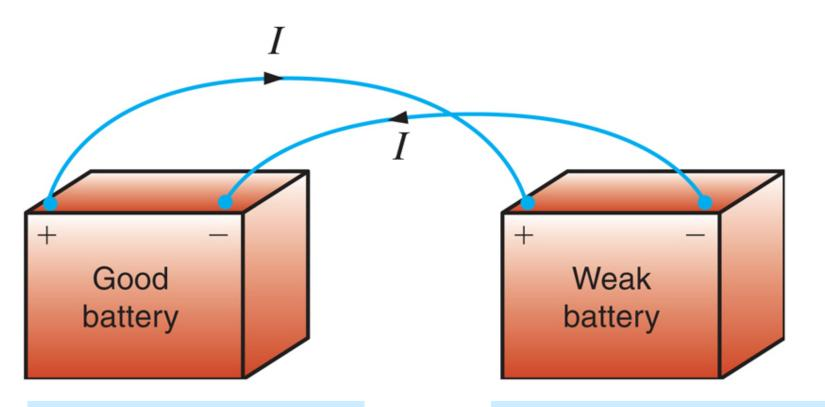
CHARGES RECEIVE ENERGY. THIS BATTERY SUPPLIES ENERGY CHARGES LOSE ENERGY. THIS BATTERY RECEIVES THE ENERGY
