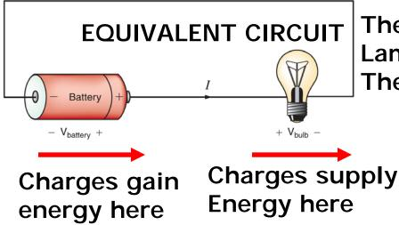
The battery supplies energy to charges. Lamp absorbs energy from charges. The net effect is an energy transfer
