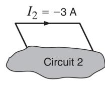
A NEGATIVE VALUE FOR THE CURRENT INDICATES FLOW IN THE OPPOSITE DIRECTION THAN THE REFERENCE DIRECTION
