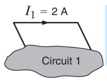
A POSITIVE VALUE FOR THE CURRENT INDICATES FLOW IN THE DIRECTION OF THE ARROW (THE REFERENCE DIRECTION)
