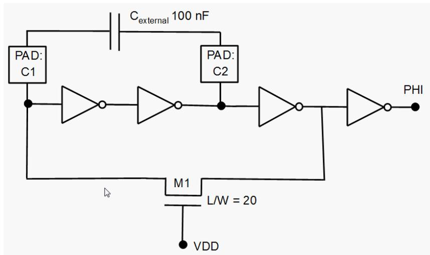
Fig. 7 Master clock generator- external capacitor  $C_{\text{external}}$  and resistance of M1 determine frequency
