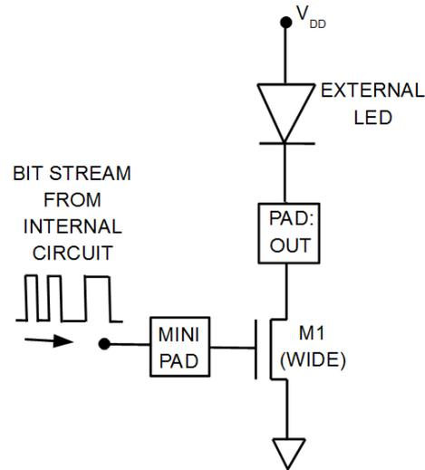
Fig. 8 Open drain output buffer
