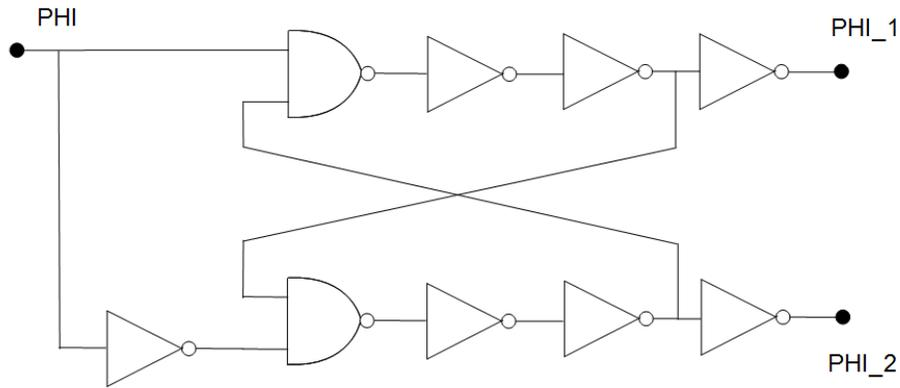
Fig. 6 2-phase clock generator **IMPORTANT NOTE CHANGE!**
