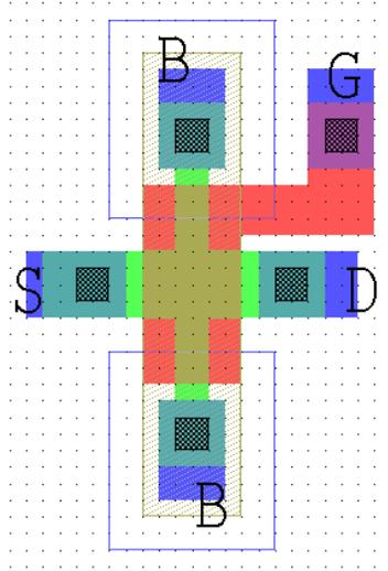
Fig. 3 Double T-gate nMOS layout for nMOS transmission gates M5 and M6 in Fig. 2.
