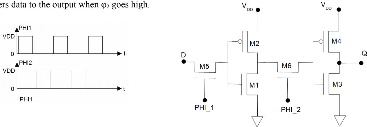
Fig. 2 Shift register stage implemented in 2-phase dynamic logic
