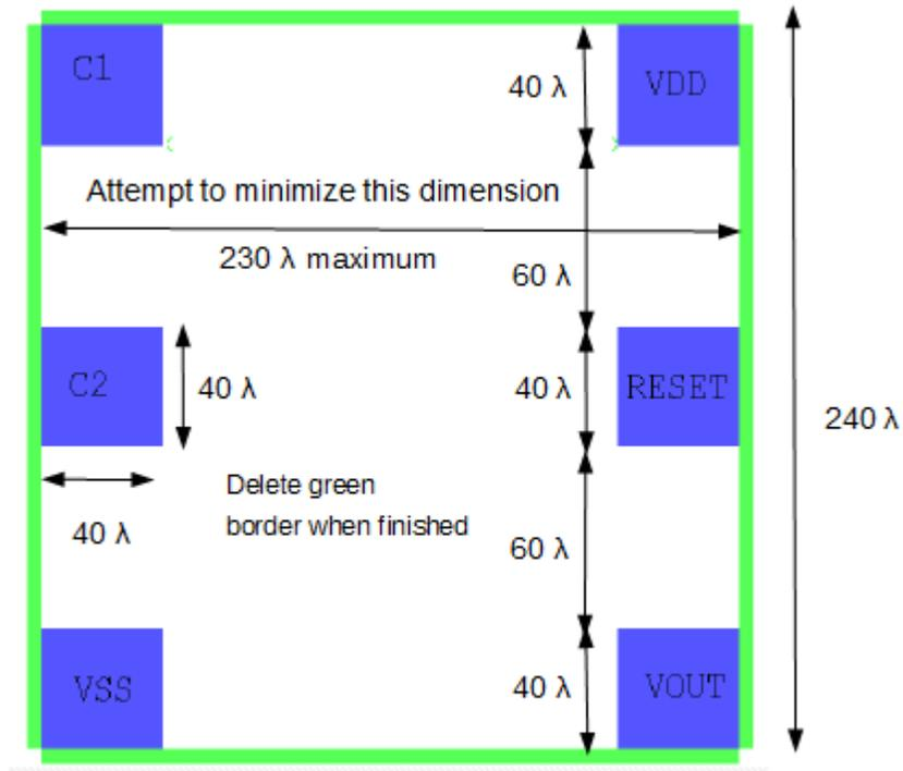
Fig. 9 Probe pad placement and available area for layout
