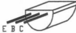
Figure 6: Lead Configuration of a 2N3904 Transistor. Lead configuration for the 2N3906 is the same.
