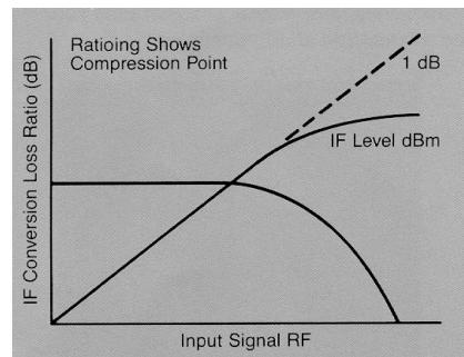
Figure 1b. Plot of conversion loss and IF output power as a function of RF input power level, note that the IF output power increases linearly with the increasing RF signal, until mixer compression begins and the mixer saturates.
