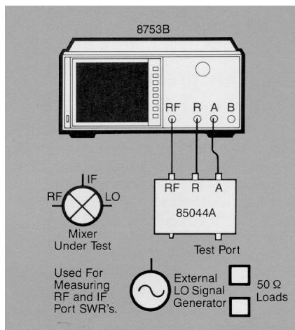
**Figure 20.** Block diagram for an SWR/return loss measurement
