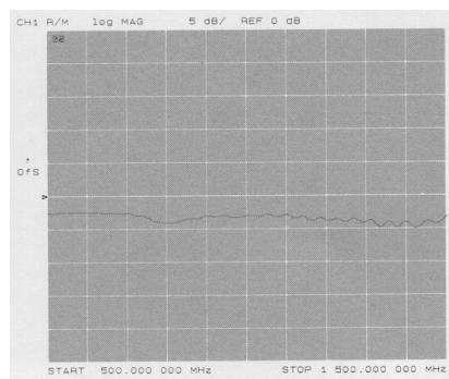
**Figure 2c.** Plot of a mixer's conversion loss vs. IF frequency neglecting attenuation at mixer ports. The frequency ripple seen is due to mixer and system port mismatches.
