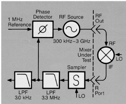
**Figure A1.** Block diagram of the 8753B receiver and a mixer under test
