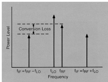
Figure 1a. Spectrum of RF, LO, and IF signals present in mixer measurements
