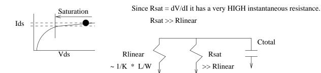
When discharging, the PMOS path is in cutoff, when charging the NMOS path is cutoff.
