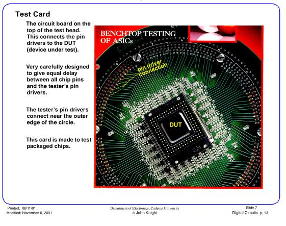
Test Card for a Packaged IC
