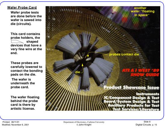
A Wafer Probe Card for Probing Die
