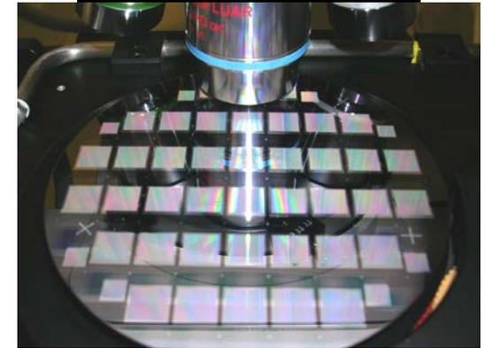
Optical microscopes are available throughout the lab for optical inspections, taking photographs and making linewidths measurements if necessary. For film thickness measurements we have ellipsometers, as well as contact and optical profilometers.. A complete 1 MHz CV test station consisting of a hot chuck with a HP4280 CV meter is available to test gate dielectric quality. A Jeol JSM840 Scanning electron microscope is available for SEM imaging.
