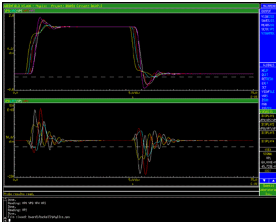
Figure 4. Illustration of cross-talk between lines due to coupling
