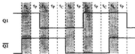
Fig. 6. Waveforms of a self-oscillating 2-bit Johnson counter with different cell delays.
