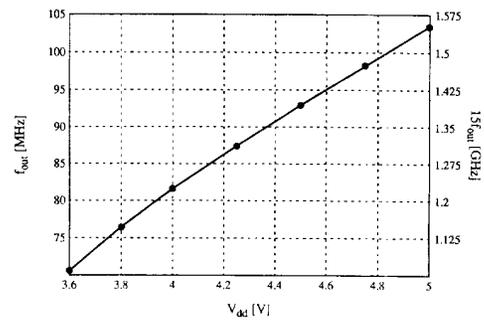
Fig. 14. Oscillation frequency as a function of supply voltage.
