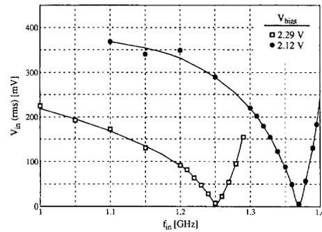
Fig. 17. Minimum required input voltage as a function of input frequency.
