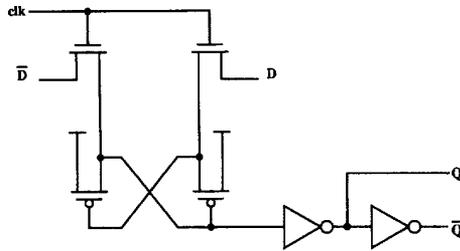
Fig. 8. Differential-logic latch.
