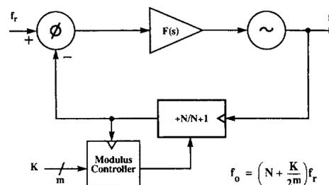
Fig. 1. Fractional-division PLL synthesizer.
