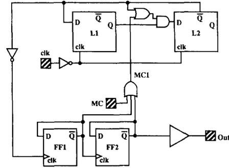
Fig. 7. Functional block diagram of the dual-modulus frequency divider.
