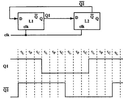
Fig. 4. A self-oscillating 2-bit Johnson counter with level-triggered latches.
