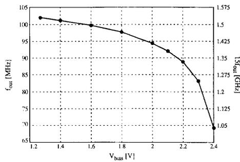
Fig. 15. Oscillation frequency as a function of bias voltage.
