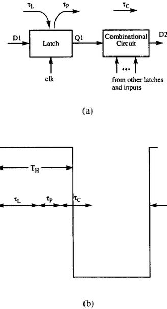
Fig. 3. (a) Block diagram of a latch-operated sequential circuit cell. (b) Positions of latch and combinational circuit time intervals with respect to the clock waveform.
