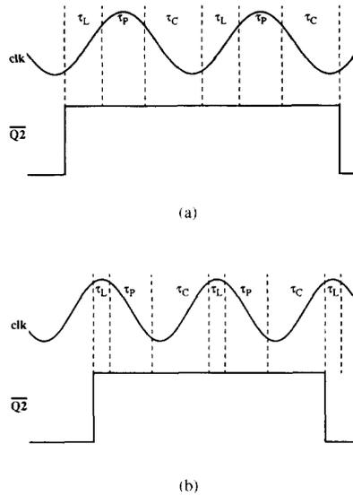
Fig. 5. (a) Input and output waveforms of a 2-bit Johnson counter with level-triggered latches. (b) The frequency divider waveforms at maximum operating frequency.
