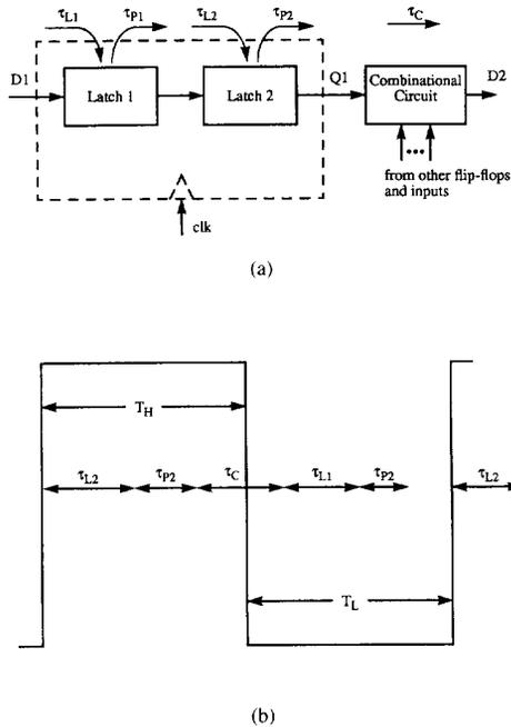
Fig. 2. (a) Block diagram of a sequential circuit cell. (b) Positions of latch and combinational circuit time intervals with respect to the clock waveform.
