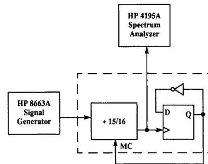
Fig. 18. Fractional-division test configuration.
