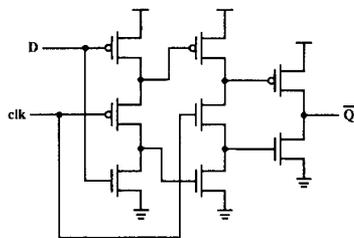
Fig. 10. Schematic diagram of the true-single-phase-clock flip-flop of the second stage.
