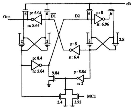
Fig. 9. Schematic diagram of the first-stage divide-by-3-or-4 counter.
