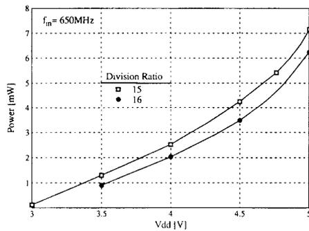
Fig. 16. Power consumption as a function of supply voltage.
