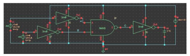
37) Now we will setup the properties of some instances. Select V0 (vdc) and press "q" to access the Edit Object Properties dialog box. In the DC Voltage field, enter **1.8 V** and click OK. Note that standard supply voltage for CMOS 0.18u technology is 1.8V.
