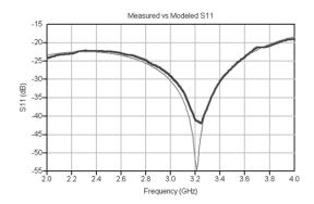
Figure 12. Comparison of S11 for the measured and modeled microstrip thru line
