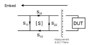
Figure 23. Diagram showing the movement in the measurement plane during de-embedding and embedding of a two-port network
