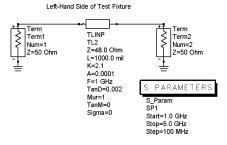
Figure 9. Agilent ADS model for the test fixture using a lossy two-port transmission line
