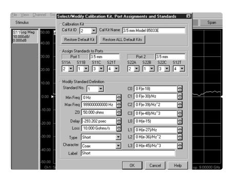
Figure 15 E8358A PNA dialog showing the modified cal kit definition
