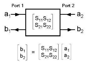
Figure 3. Definition of a two-port S-Parameter network
