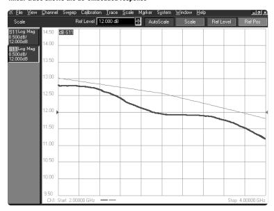
Figure 21. Measured S21 of a surface mount amplifier. The lower trace shoes the response using a standard coaxial calibration and the upper trace shows the de-embedded response
