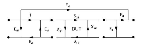
Figure 17. Signal flow diagram of the forward two-port error terms
