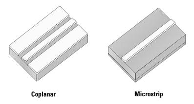
Figure 1. Types of printed circuit transmission lines
