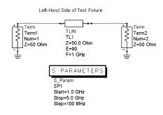
Figure 7. Agilent ADS model for the test fixture using an ideal two-port transmission line
