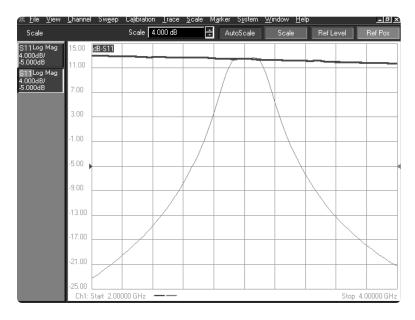
Figure 24. Measured S21 showing the effects of embedding a virtual bandpass filter network into the measurement of a surface mount amplifier. Upper trace is the measured response of the amplifier only. Lower trace shows the response including an embedded filter network
