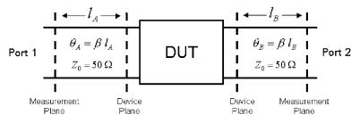
Figure 6. Modeling the fixture using an ideal transmission line
