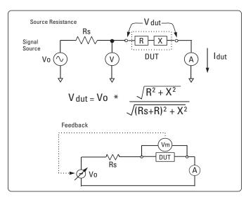
Figure 2-3. Applied Signal and Constant Level Mechanism
