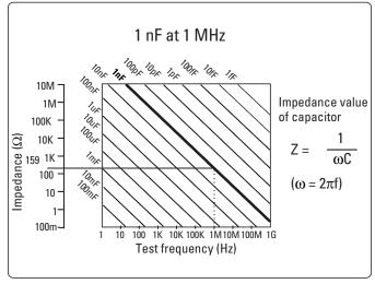
Figure 4-1. Capacitor Impedance and Test Frequency
