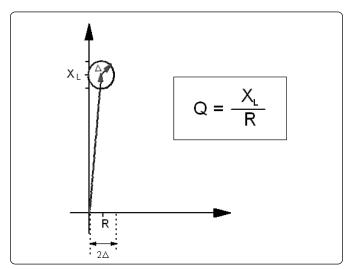
Figure 4-2. Concept of the Q Error
