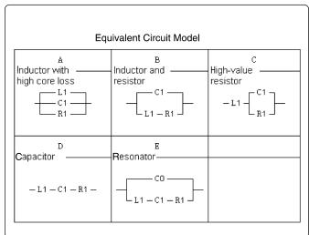
Figure 3-2. Equivalent Circuit Analysis Function
