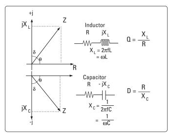
Figure 1-2. Capacitor and Inductor Parameters
