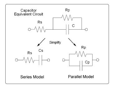
Figure 3-1. Measurement Circuit Mode
