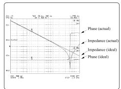
Figure 2-1. Frequency Characteristics of a Capacitor
