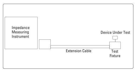
Figure 7-1. Measurement Port Extension
