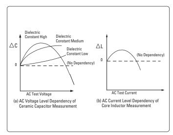
Figure 2-2. Signal Level Dependency
