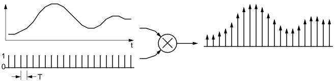
In the frequency domain, the series of pulses in the time domain is equivalent to an infinite series of pulses in the frequency domain separated by 1/T.
