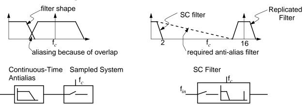
The systems view is shown on the left. The commonly quoted rule for this system is: - Filter shape should not extend past  $f_c/2$ , then there will be no aliasing. This is very important when trying to design
