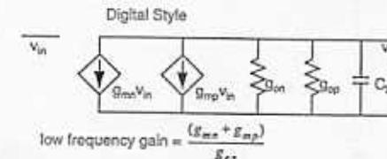
$$\text{low frequency gain} = \frac{(g_{m1} + g_{m2})}{g_{eq}}$$
