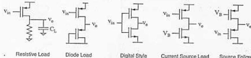
$$\frac{V_o}{V_{in}} = \frac{g_m}{g_{d1} + g_{d2}} \quad \frac{V_o}{V_{in}} = \frac{g_{m1}}{g_{m2} + g_{d11} + g_{d12}} \quad \frac{V_o}{V_{in}} = \frac{g_{m1} + g_{m2}}{g_{d11} + g_{d12}} \quad \frac{V_o}{V_{in}} = \frac{g_{m1}}{g_{d11} + g_{d12}} \quad \frac{V_o}{V_{in}} = \frac{g_{m1}}{g_{m1} + g_{d11}}$$
